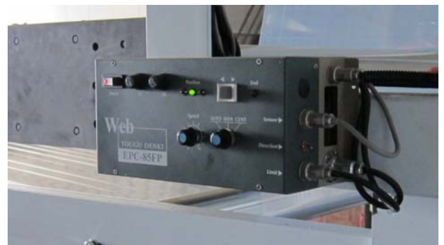
Controller 85FP is installed on Blown Film Machine by Wall-Mounted
